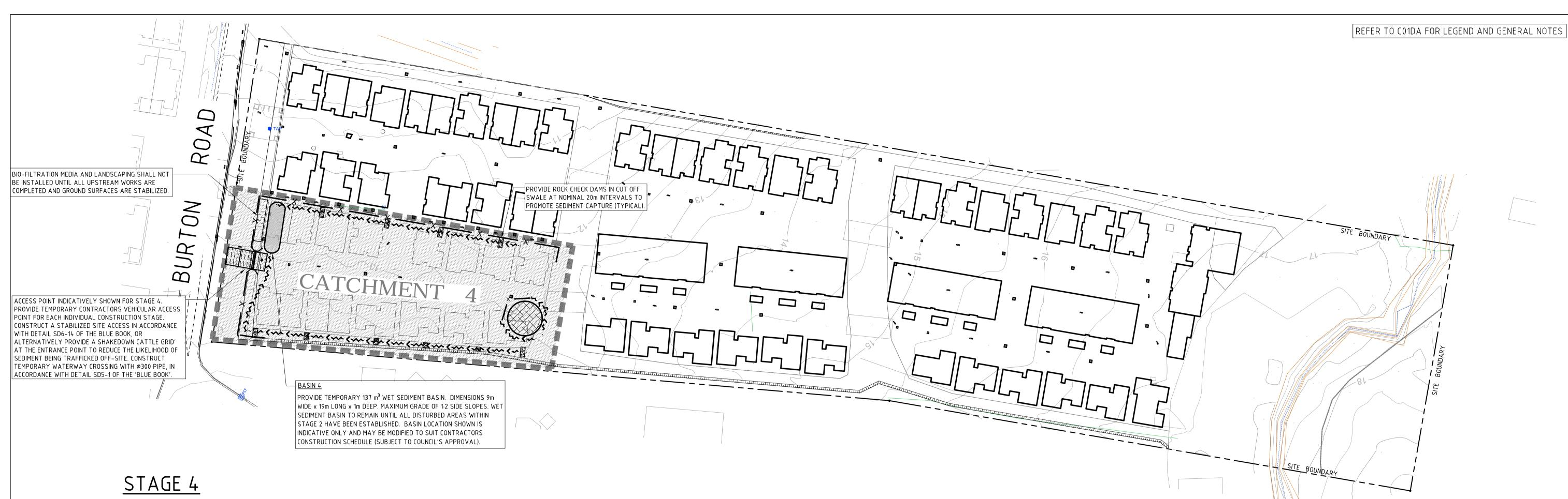
CONCEPT SEDIMENT & EROSION CONTROL PLAN
